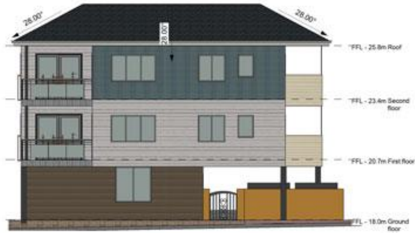
1 Apartment South elevation 1 : 100
