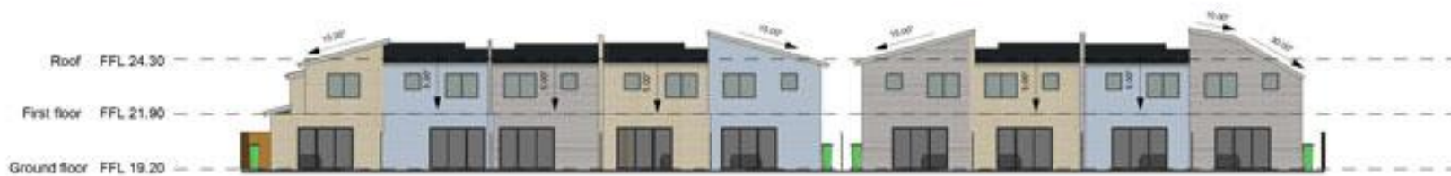
1 terrace house east elevation 1 : 200
